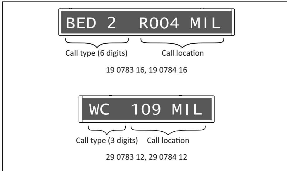
Fig. 6: Signalling on the corridor displays
